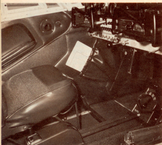
Cockpit of the Cherokee 235 features recessed arm rest, which adds cabin width, map pocket and an instrument panel designed to accommodate full instrumentation for IFR flying. In the center area, between the seats are (left to right): flap handle, fuel-tank selector valve and brake handle center-mounted under the throttle
