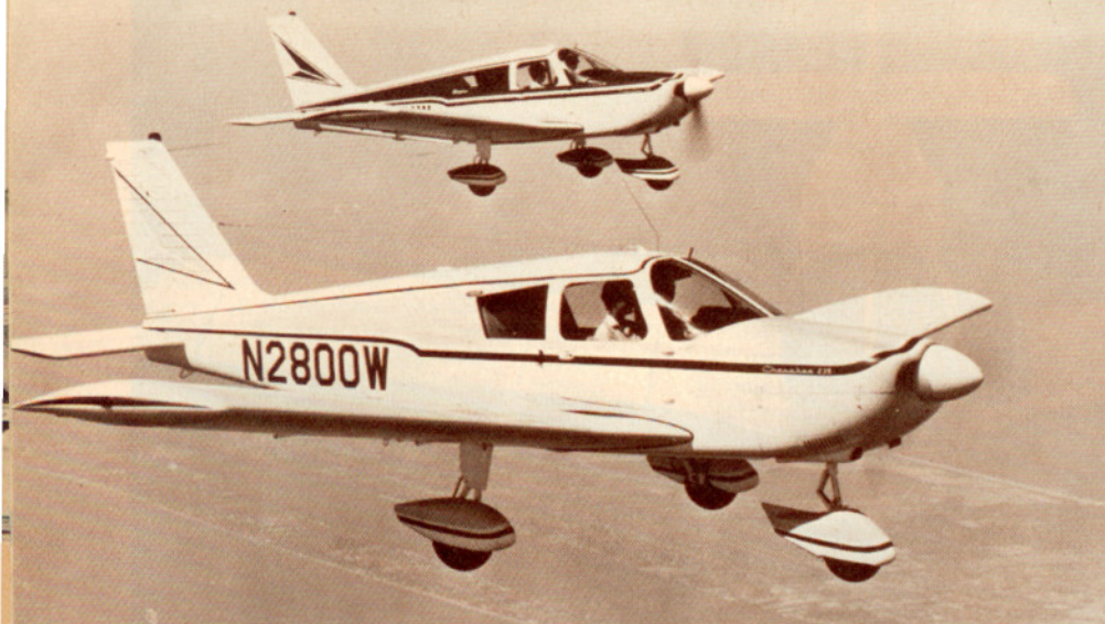
Piper's new 235 h.p. Cherokee will carry a useful load 80 pounds greater than its empty weight (1,410 pounds). Greater wing spread and sculptured cowl distinguish the 235 Cherokee from its Cherokee B stablemate, which is offered with 150, 160 or 180 h.p. engines. The new plane will carry four 170-pound passengers, 84 gallons of fuel, 200 pounds of baggage, full instruments and radio with weight allowance left over
